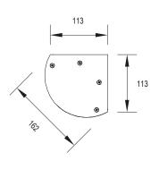
Angled LED fitting with a slim-line curved profile capable of continuous mounting (cable runs can be housed within angled back body).
