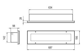
Recessed linear LED fitting, unique upstand recessing flange, suitable for new installations or retrofitting into existing cavities when Bergo, Bergen or Victor have been removed.
