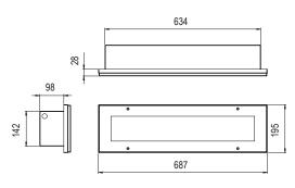
Recessed linear LED fitting, unique upstand recessing flange, suitable for new installations or retrofitting into existing cavities when Bergo, Bergen or Victor have been removed.
