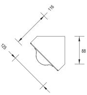
The 'tough brother' of the Forum, designed for installations where severe or prolonged attack may occur. Angled body in zinc coated steel.
