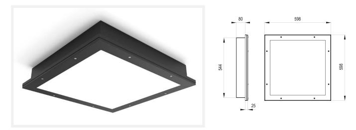
Square recessed body manufactured from zinc coated steel with upstand recess. Mounting through body sides to ceiling frame or through rear of body dependent on ceiling type. 3mm clear patterned polycarbonate flat panel secured by anti-tamper fixings.
